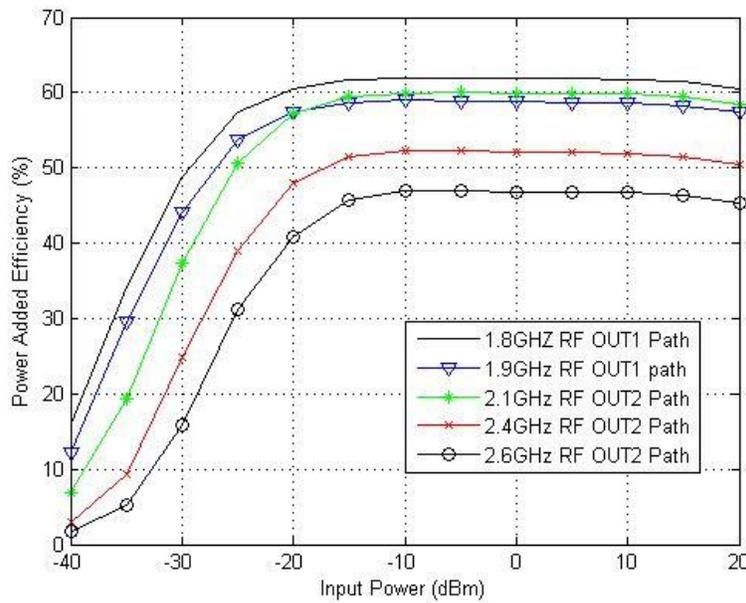
**Figure (10):** Simulated PAE versus input power at 1.8/1.9/2.1/2.4/2.6 GHz
