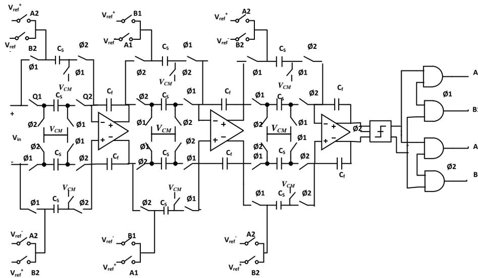
Figure (3): The 3<sup>rd</sup> order switched capacitor LP ΣΔ modulator
