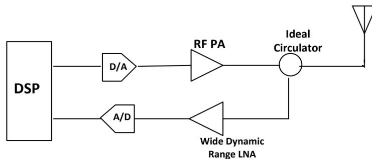
**Figure (1):** Ideal software SDR transceiver architecture
