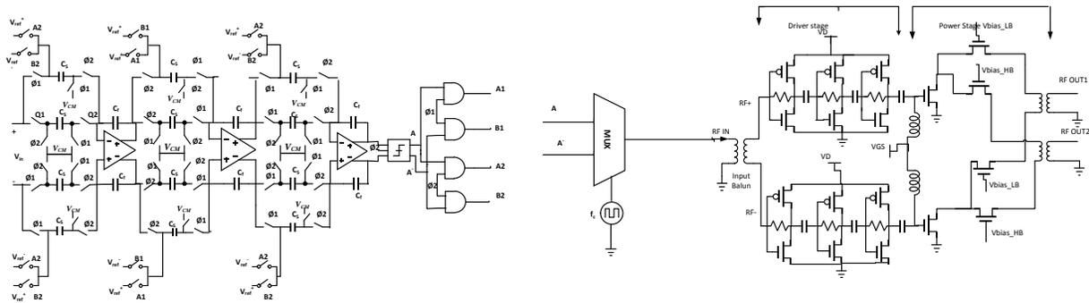
**Figure (11):** Complete schematic of LP  $\Sigma\Delta$  transmitter driving a switching mode class E PA
