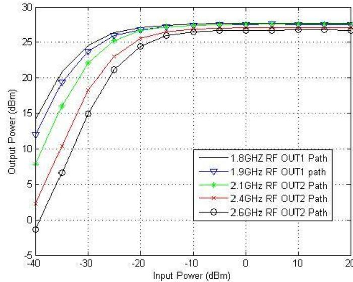
**Figure (9):** Simulated output Power versus input power at 1.8/1.9/2.1/2.4/2.6 GHz
